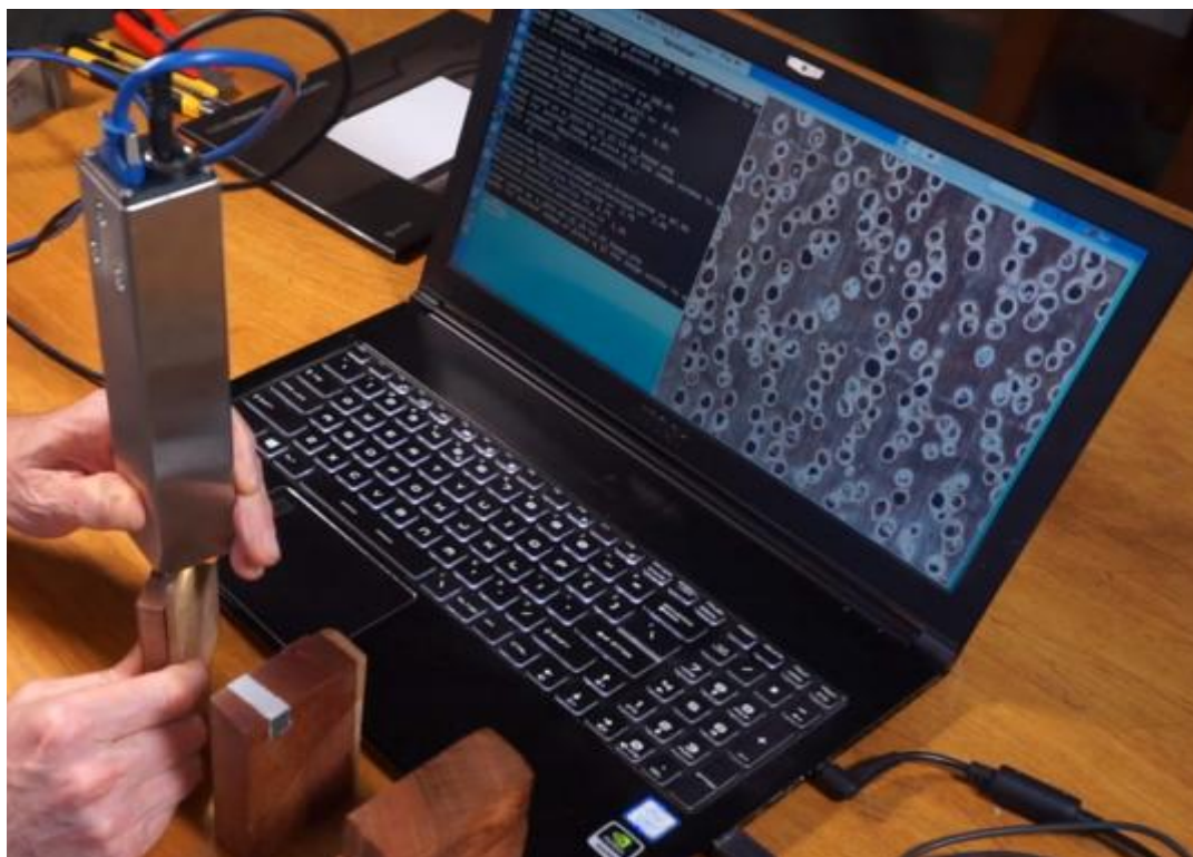
Figure 14. Example of the XyloTron machine-vision based system usage, scanning a transversal section of a piece of timber for its identification. Source: https://www.xylotron.org/index.htm
