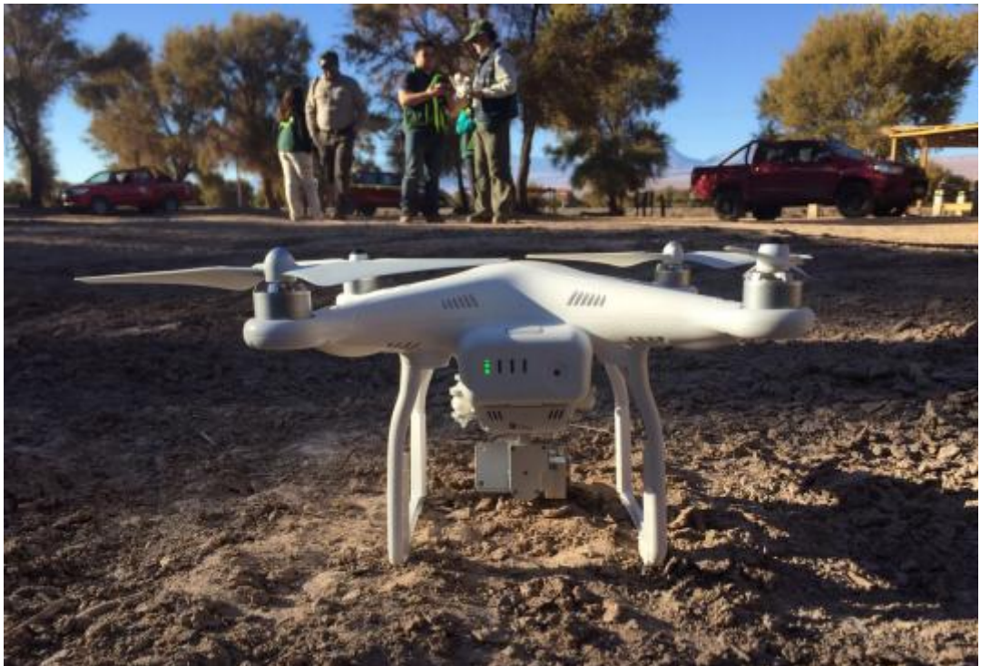
Figure 9. DJI Phantom 4, a low-cost UAV option for forest surveillance and evaluation. Source: CONAF (Chile).
