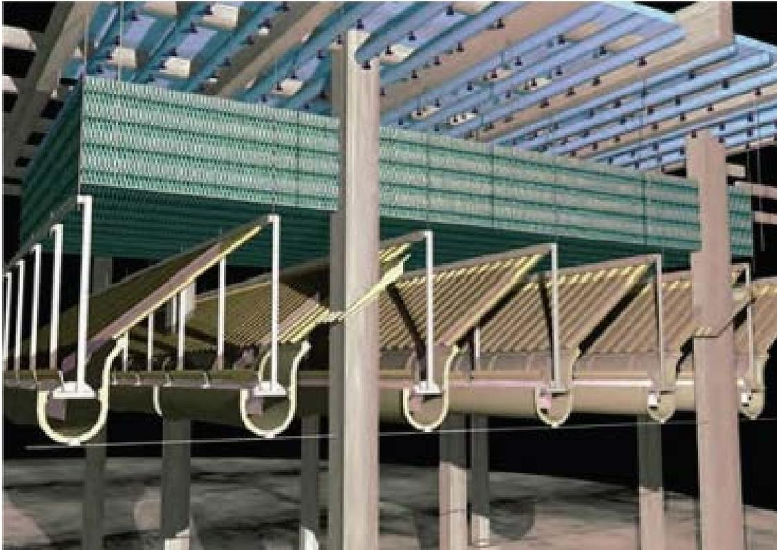
Figure 4 – Anqing High-Yield Wet Cooling Tower Internal Structure<sup>3</sup>
