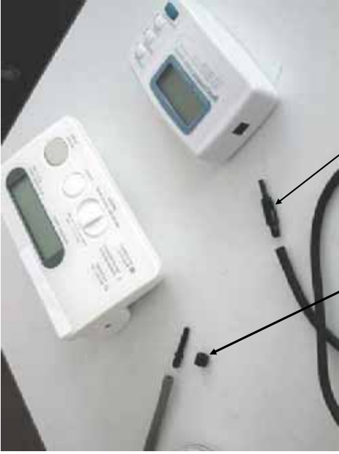
Configuration for normal use, disconnected plug; upper part: removed spacer, downer part: turned plug
