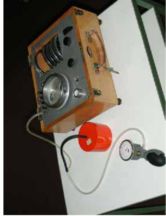
Figure: Measurement setup to determine the limits of error of the cuff pressure indication (aneroid manometer)
