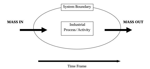
A mass balance can be undertaken to varying degrees of precision and depth. In evaluating eco-efficiency opportunities for small and medium sized companies, it is prudent to limit the detail of the initial
