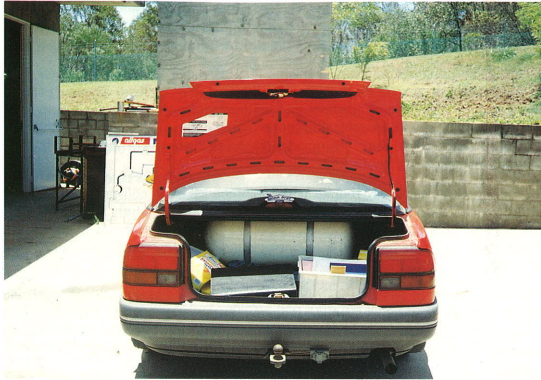
An NGV showing on board storage.
