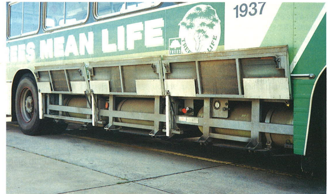
An NGV bus showing on board storage.
