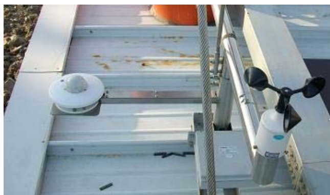
Figure 4-41 Irradiator Blocked By Shade
