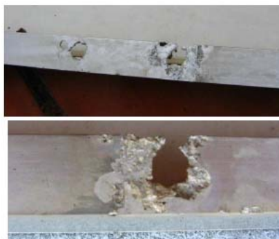
Figure 4-15 Module Problems Caused by Salt Mist and Ammonia Gas
