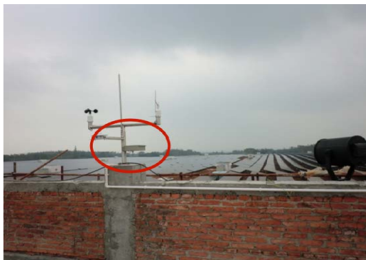
Figure 4-43 Inclined Environment Monitoring Instrument Holder
