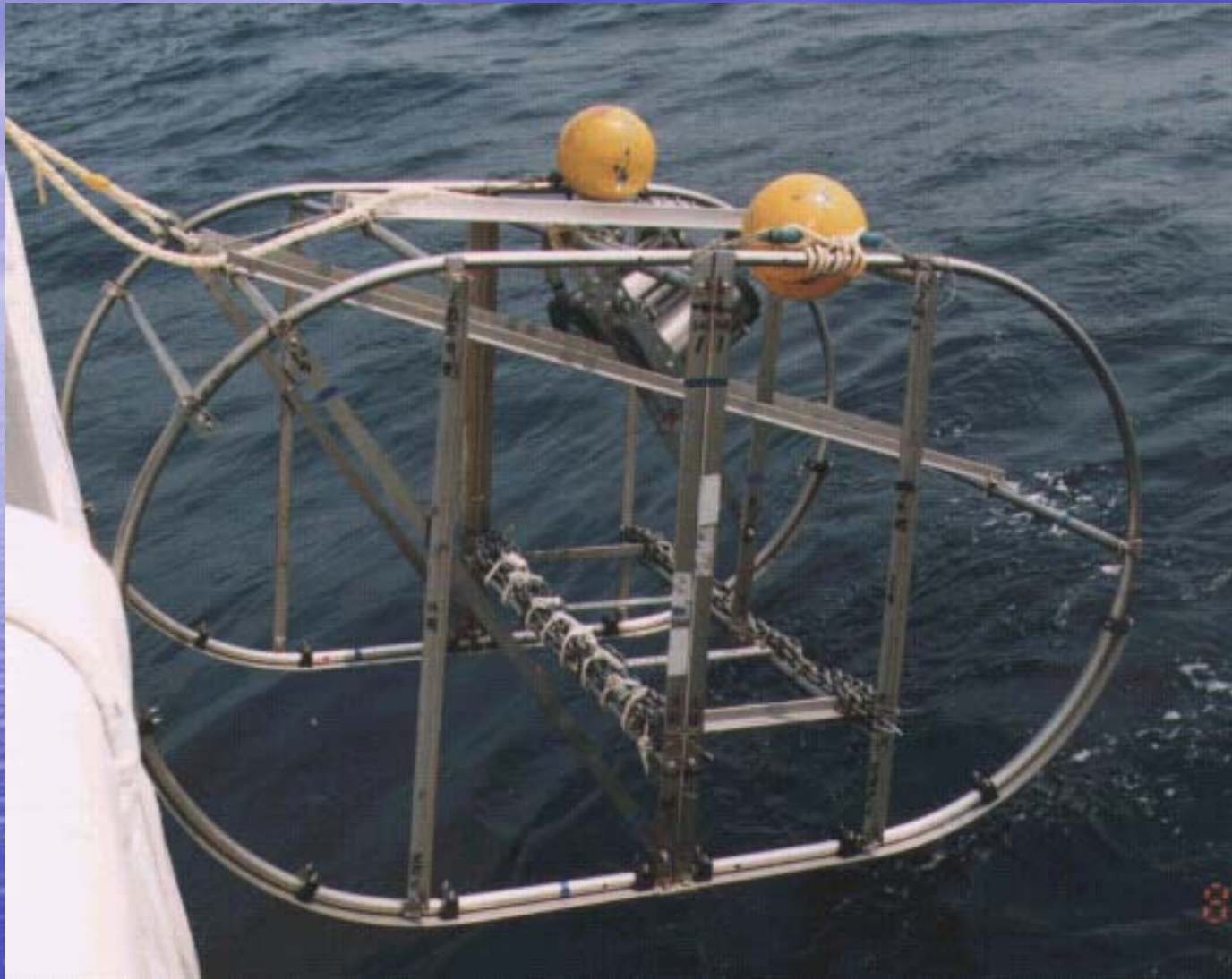
Deep-sea Video Monitoring System on a Towed Sledge (DVMSTS)
