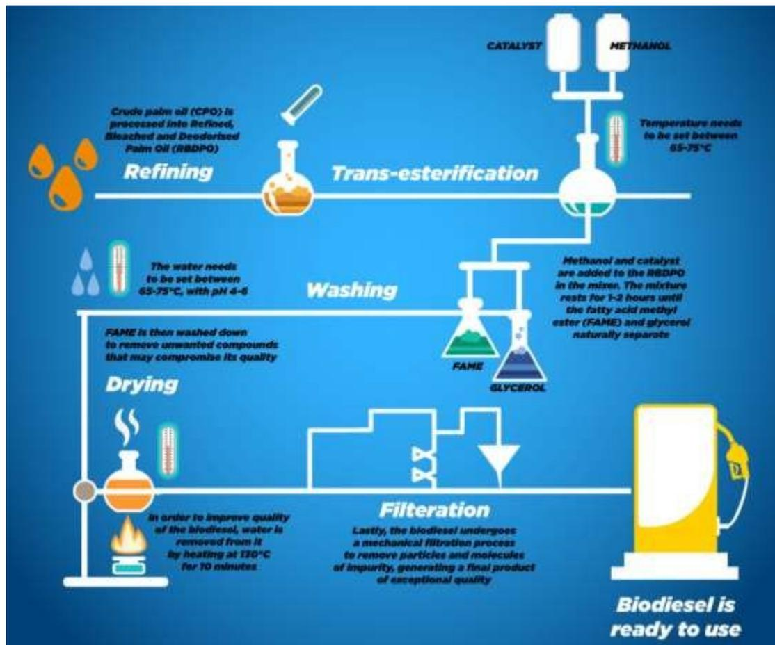
Figure 7: Malaysia biodiesel production process (Chin, 2019)
