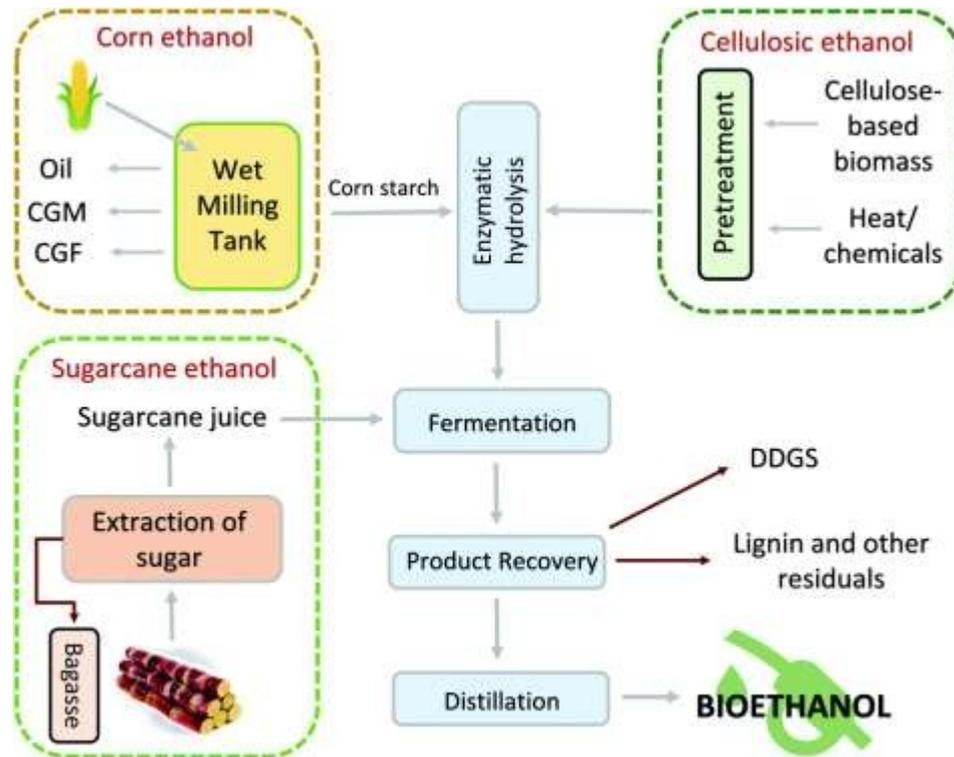
Figure 3: Bioethanol production process (Gavahian et al., 2019)
