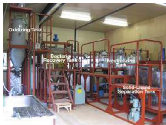
Figure 4.11 Test of sludge reduction at Horobetsu Sulfur Mine (Hokkaido Prefecture)
