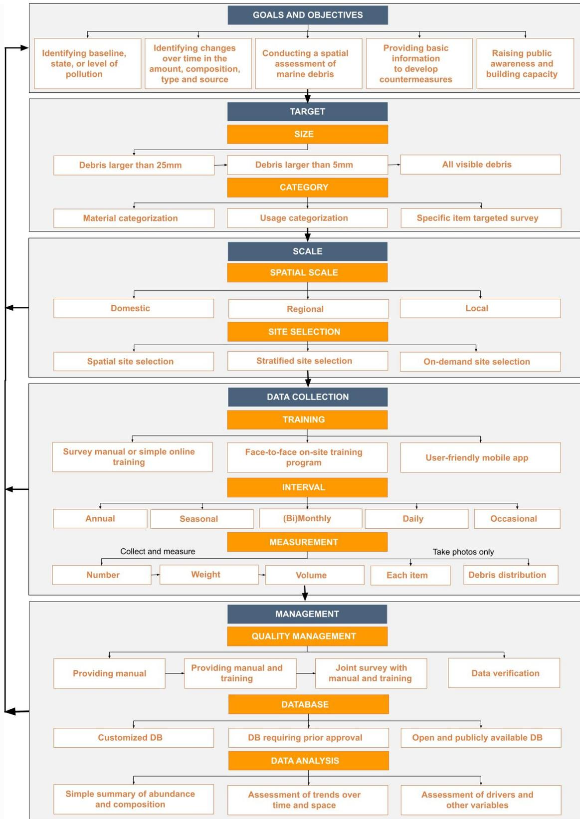
Figure 2. Decision flowchart for developing a shoreline marine debris monitoring program. The order of criteria can be changed according to the users' intention.
