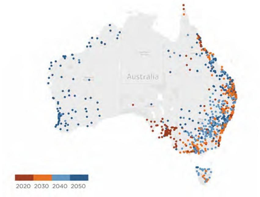
Figure 4-9. Distribution substations in Australia projected to experience reverse power flow from rooftop solar [37]
