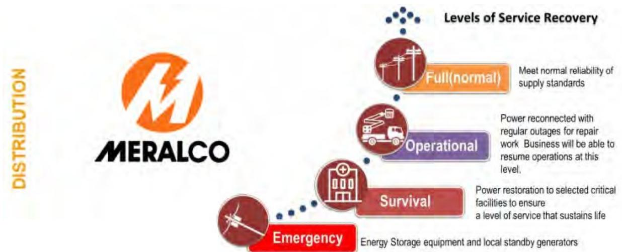
Figure 4-49. Manila Electric Company (MERALCO) post-disaster recovery process for the distribution system [131]
