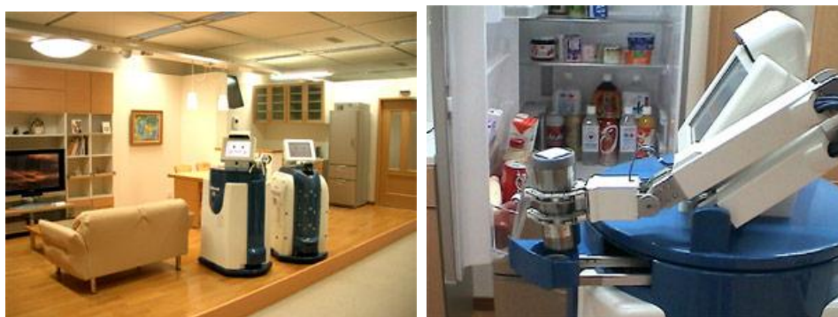
Figure 7: Coordinated operation among a life-supporting robot system (RT space), a refrigerator and a mobile robot 38
