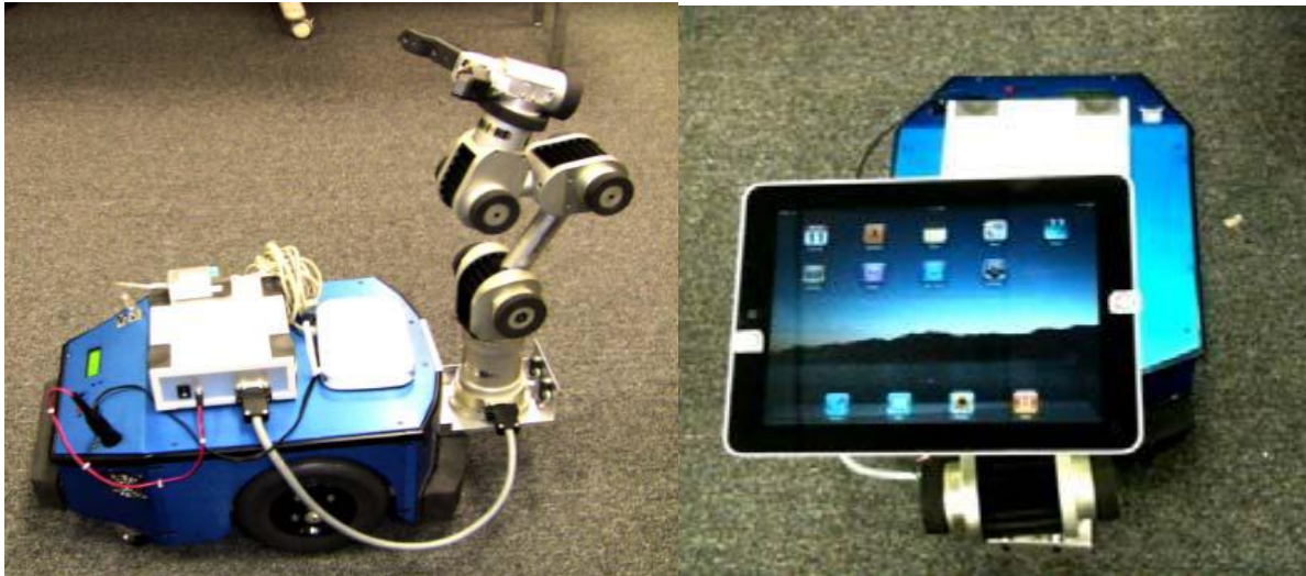
Figure 6: Neptune with iPad and Flexi Force sensors mounted on the iPad Tablet 100
