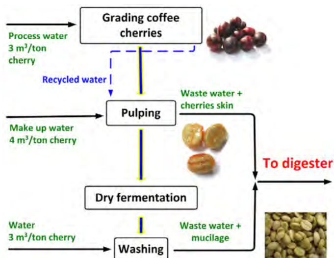
Figure 1. A schematic of fully washed method of coffee processing.
