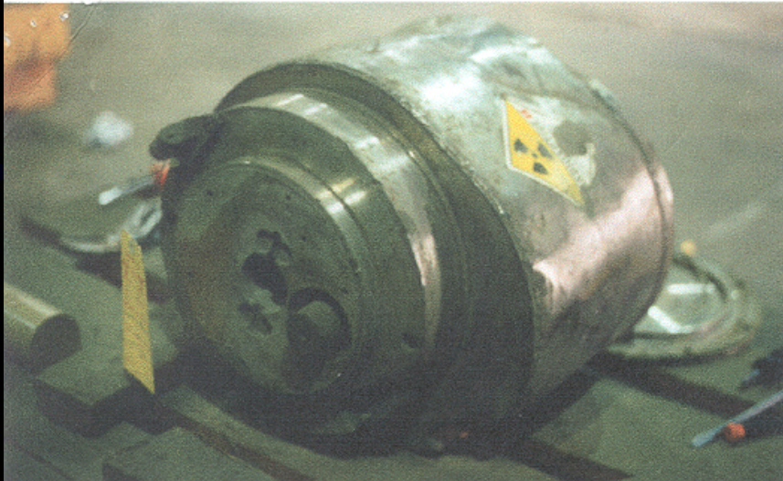
Depleted uranium caske filled with cobalt 60
