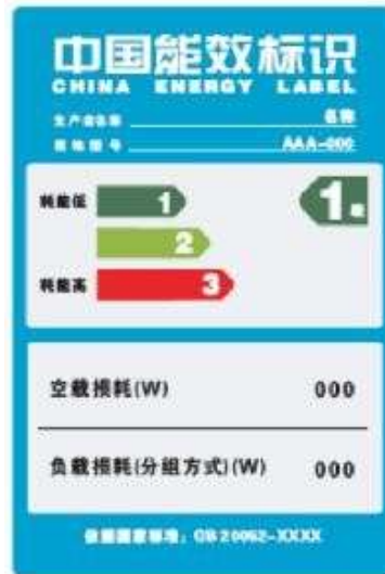
Figure 4.4 Pattern of China energy label of three-phase distribution transformer
